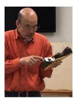
**Steve Kelem** described how he made footstool legs of poplar using a CNC turning center. The leg has a square top portion to receive the rails that are joined to the leg with Festool's domino floating tenons. The next section is round that contains half rounded flutes while the next two lower sections are tapered. The bottom section is a straight cylinder.
