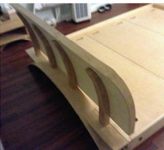
The headboard substrate is made of four layers of wiggle board overlaid with maple door skins that were covered with the outside maple veneer then pressed in a vacuum bag. The veneer split and curled up the first two times the veneer was applied and had to be removed. Two sheets of glue made in
