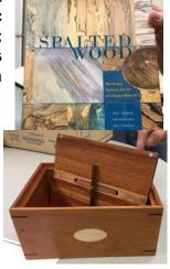
He brought in two boxes each made from one piece of Baltic birch where the sides were folded
