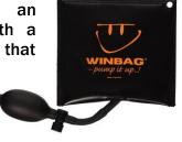
attached that when squeezed will inflate the bag. A rubber hose between the bag and bulb has an on-off valve to maintain pressure when in use. It's called a "Winbag" and is available at Amazon.com for \$18.00. AirShim is another brand.
