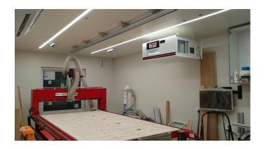
**Steve Kelem** brightened his shop with two LED strip lights. The lights come in 20 foot rolls, but he only used 16 feet of each strip. The strips are rated 24 volts, and consumes 6.6 watts of power per foot.
