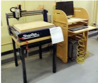
The ShopBot has a large table of particleboard where the material to be cut is attached with brass screws. The router is suspended above the table on a gantry that allows the cutter to move
