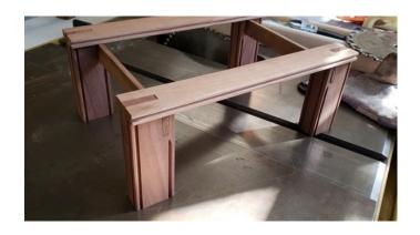
Jeff Lukanc created two stands for his laptop computer with one made from koa and the other made from teak. One is for home and the other is for his office. It's made with finger joints and contains no screws. The middle is left open and acts as a cooling vent for the computer. Jeff used Freud's box joint cutter set of saw blades for the joints. Placing the blades back to back produces a 1/4" cut and placing the blades front to front produces a 3/8" cut.
