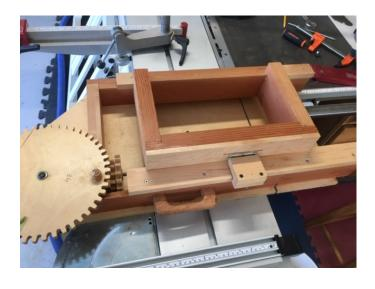
**Bill Henzel** showed us a jig for making 1/8" finger joints using a saw blade with a square-topped surface grind. The box on top allowed him to cut multiple pieces at once by offsetting every other one an eighth of an inch. He used the jig to make a mahogany sewing box. Six boxes sit on top of the base and swing out to reveal the contents. The handle is a bent lamination clamped over a form with each quarter-sawn slat measuring .048 inches thick.
