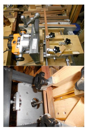
Ron Gerard made a horizontal mortiser featuring a 3 1/4 hp Triton router. The three axis's all run on sets of linear bearings. It typically uses a ½" cutter, but 3/8" and ¼" cutters can also be used with bushings. It creates a large amount of chips and the next step is to add a dust collection port.
