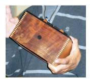
A second box sports finger joints made with the jig that he demonstrated in last month's program. It's made of maple,
