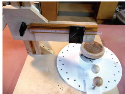
A plate jig for making miniature bowls was discussed along with individual segment placement jigs which allow more flexibility in placing the segments. The jig that Tom uses was based on those made by others using a plate for 16 segments with an 8 degree gap.
