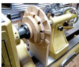
He defined the terminology involved such as angles of cut and steps in cutting the segments using a "wedgie sled".
