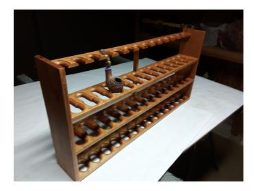
**Syd Dunton** made a pipe rack of cherry that measures 30 inches wide by 4 1/2 inches deep and has spaces for 28 pipes. The keyhole shaped holes are two inches on center. Because the rack is so wide, he placed a vertical support in the middle. The project is finished with polyurethane.
