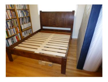
Dennis Yamamoto created a queen sized bed from claro walnut. The frame of the headboard is constructed using loose tenons in mortice and tenon joints. The panels in the headboard are made up of four laminations. He used both Unibond and epoxy glues. The horizontal slats are maple except for two. He used what he had on hand and came up short so he used mahogany pieces to fill in.
