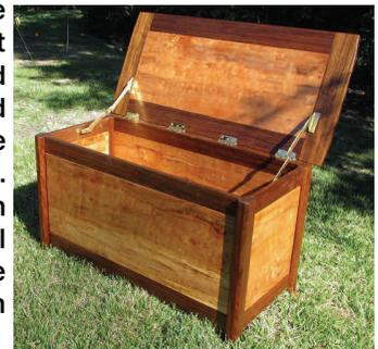
page 38. The lid is held open by heavy duty hardware he made from 1/8 inch sheet brass with brass rivets made from 1/4 inch brass rod.
