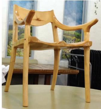
**J**eff Yen, working in Fred Sotcher's shop for close to a year, created a Sam Maloof style chair. It's made from figured English sycamore with contrasting wood to cover the screw holes and finished with polyurethane. He described how the joints were made and discussed some of the problems encountered.
