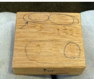
**T**erry O'Donnell presented some examples of repaired wood as discussed in the March meeting. A recess is gouged where the patch is needed then another piece is gouged in matching material using a deeper cut to create a
