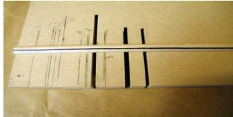
For small boxes, Mike uses five segments for the hinge with the middle three segments being drilled all the way through and the two end segments drilled only part way through from one end.
