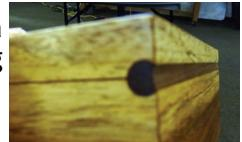
The dowel diameter must be the same thickness as the project material. The minimum dowel diameter is 3/8" although 1/2" is a better size to work with. The tools and materials needed to make the box hinge are 1/8" brass rod and brad point drill, a cove router bit the same diameter as the dowel that is used, blue tape, glue, paste wax, A special drill bushing that's internally tapered from the size of the dowel down to 1/8".
