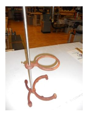
**Alan Kutach** made a pour-over coffee pot support stand from ironwood and eucalyptus with a steel rod. He uses the support stand every day. The base and support ring were cut with a CAD router.
