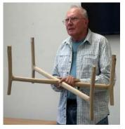
month, he brought in the base with horizontal members crossed at 45 degrees using a lap joint. He used mortise and tenon joints between the horizontal and vertical members and all pieces are rounded by a 1/2" round-over bit installed in a router table. He then worked it over with an orbital sander. The top and base will not be permanently attached to each other for ease in moving the table about.
