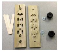
project at the Maker Faire. The project is a scissor jack. The jig is made of two pieces of poplar where one side has formed pegs while the other side has corresponding holes. T-bolts were placed at either end to clamp the two halves of the jig together. Both sides were cut on a CNC machine.
