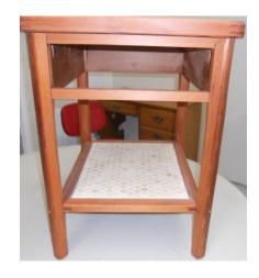
The joints are mortise and tenon and the legs are shaped with files and a spoke shave. An exterior oil will be applied as a finish. There will be two similar tables made for inside the house using black walnut instead of redwood.
