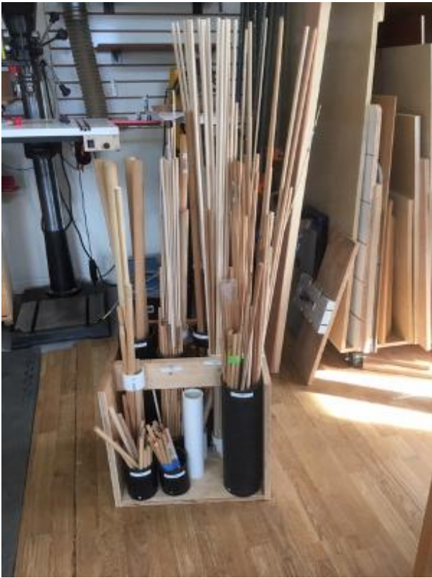
Bill Henzel organized his collection of dowels by using various sizes of ABS and PVC pipe attached to a plywood box. They are loosely segregated by length.
