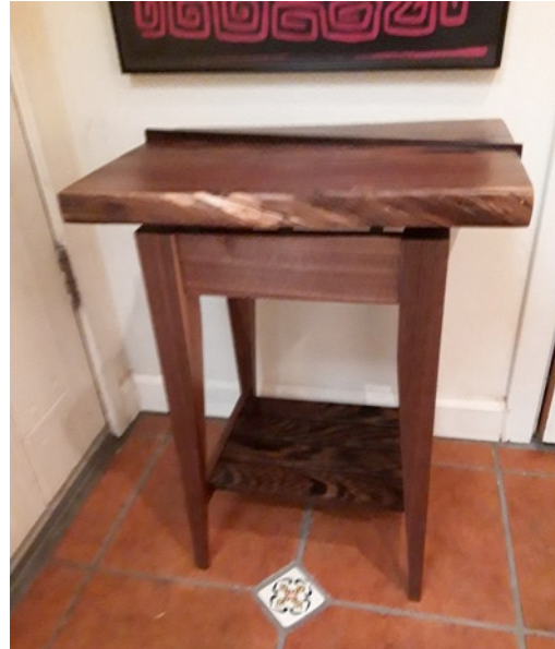
Syd Dunton made a small table of eastern and claro walnut with accents of wenge. It measures 19" tall, by 22" wide by 14" deep. The shelf is wenge. Walnut is used for the top and is raised and supported with pieces of ebony. The top also features a slat of wenge that slashes diagonally across the table top in a sloping angle.
