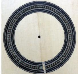
can be identified by their rosettes. He glues the rosettes to the body before the hole is routed in the center using an aluminum jig attached to the router base.
