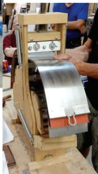
Tim demonstrated how the body sides are formed. The two sides are formed separately on a jig where the side being formed is pressed into the proper shape. An electric
