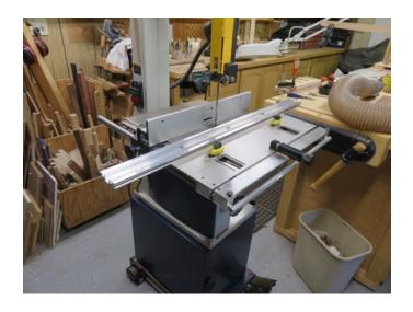
The first jig I demonstrated was Accu-Slice, <a href="http://www.accu-slice.com">http://www.accu-slice.com</a>, which provides an accurate way of resawing wood with the bandsaw. The Accu-Slice base attaches to the bandsaw table,
