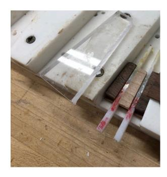
The in-progress bowl has 70 5-piece segments. I showed the jig used as an assembly aid for these segments.
