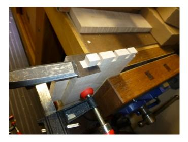
He also showed us a simple jig for paring the shoulder of a board when cutting the tails on a dovetail joint. Jim Budlong of the Krenov School came up with this idea.
