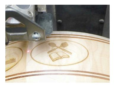
The laser acts just like a computer printer with laser unique parameters set in printer setup. For engraving the laser power and speed are specified which vary according to wood and desired engraving dept. For each segment, the laser pointer was set to the
