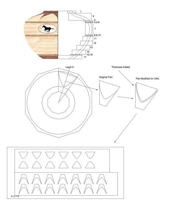
Once the bowl's profile and layers are designed, the layer 2 parts are detailed. In some cases, the part design needs modification if the CNC is used. In this case, thickness is added to the base, allowing additional material for sanding to get crisp scallop points. These modified parts are placed on a separate drawing, replicated, arranged to fit the material, oriented appropriately, and router bit clearance accommodated. It is this drawing that is exported to the CNC.
