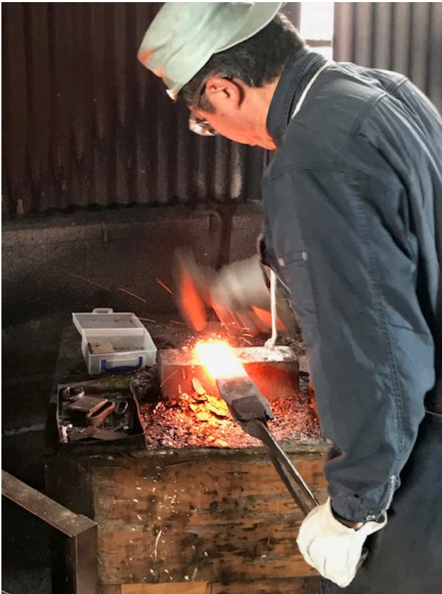
Forging a plane iron. Japan, 2017 Jay Perrine
