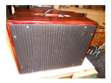
Eugene also brought in a full-range speaker that he uses with his guitars. He made it from pine to keep the weight down because of the heft of the speakers. He cut box joints using an Incra Jig at the corners for strength and will add metal caps at the corners to reduce damage. The enclosure is colored burgundy and is finished with Minwax polyurethane.
