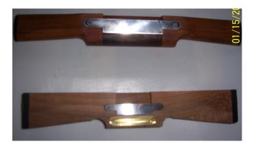
Both bodies are made from apricot wood with ebony end caps for contrast. The larger tool has an ironwood insert behind the blade to deal with wear. The smaller shave's body is still in the roughed out stage. It has a brass strip imbedded behind the blade to deal with wear.
