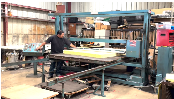
Horizontal bandsaw cutting foam
