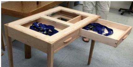
described its construction. It has two unique drawers that slide out either side of the table. The top
