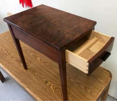
The back and side rails are veneered using 1/2" Baltic birch plywood with 1/8" walnut panels on either side of the plywood. Before the walnut panels were glued to the
