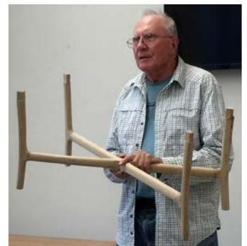
month, he brought in the base with horizontal members crossed at 45 degrees using a lap joint. He used mortise and tenon joints between the horizontal and vertical members and all pieces are rounded by a 1/2" round-over bit installed in a router table. He then worked it over with an orbital sander. The top and base will not be permanently attached to each other for ease in moving the table about.
