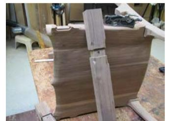
Many chair joints are not at right angle to each other and Chuck has found that using a 12" disk sander is the best way to ensure the mating
