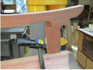
Chuck cautioned us that the pieces should be left oversized until all the joints are mated properly.
